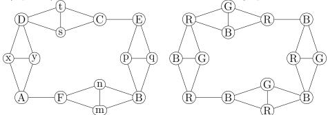
**Solution:** The chromatic number is three. The picture above shows that it can be colored with three colors (upper bound). Since it contains triangles, we also have a lower bound of three.
