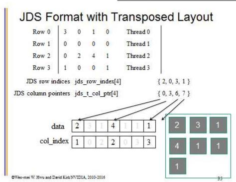
(A) In the following JDS\_T kernel, fill in the missing indexing expressions for accessing data (input matrix), x (input vector) and y (output vector).
