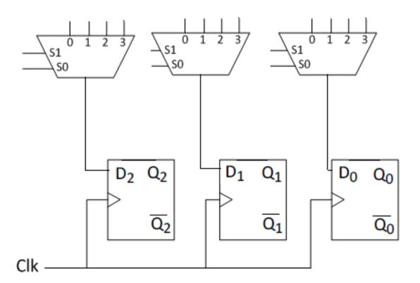
2. (2 points) If the shift register initially stores Q<sub>2</sub>Q<sub>1</sub>Q<sub>0</sub>=101, what is stored in the register after one clock cycle when AB=10?
