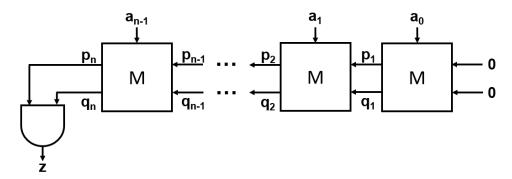
**1. (8 points)** Give meanings to each combination of the carry bits  $p_{i+1}q_{i+1}$  in the table below, so that they are **consistent with the diagram above**. One meaning has been provided to you.
