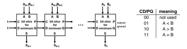
Your ECE120 lab partner suggests that rather than implementing the bit slice from gates, one can use a comparator bit slice and a mux, as shown below. The representation used for bits between comparator bit slices is the same as the representation used between the bit slices being implemented, as shown to the right.
