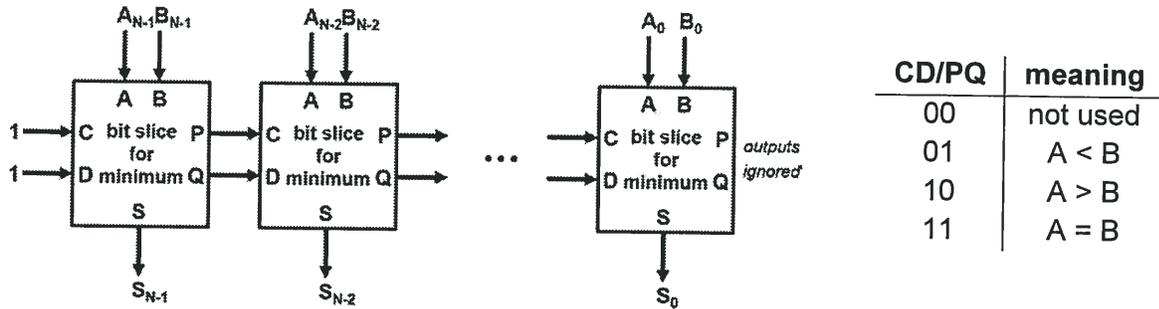
Your ECE120 lab partner suggests that rather than implementing the bit slice from gates, one can use a comparator bit slice and a mux, as shown below. The representation used for bits between comparator bit slices is the same as the representation used between the bit slices being implemented, as shown to the right.
