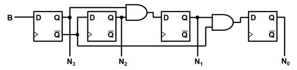
Assume that  $N_3N_2N_1N_0$  are unknown at the start of operation (that is, in clock cycle 0) and that input B is set to the sequence 0, 1, 0, 1 (from clock cycle 0 to 3). Fill in the values of  $N_3N_2N_1N_0$  for clock cycles 2 to 4 in the table below. If a particular bit's value is not possible to know, write "unknown."
