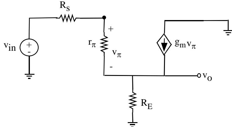
$$v_o = \left( g_m v_\pi + \frac{v_\pi}{r_\pi} \right) R_E = v_\pi R_E \left( g_m + \frac{1}{r_\pi} \right)$$
