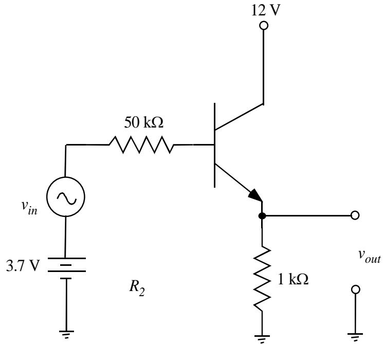
Part (b),  $R_S = 50 \text{ k}\Omega$ ,  $V_S = 3.7 \text{ V}$
