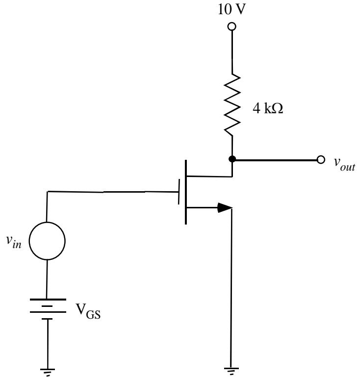
$$I_D = \frac{\mu C_{ox} W}{2L} (V_{GS} - V_T)^2 [1 + \lambda V_{DSQ}]$$
