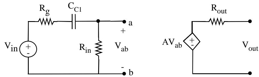
$$\frac{V_{ab}}{V_{in}} = \frac{R_{in}}{R_{in} + R_g + 1/j\omega C_{c1}} = \frac{R_{in}/(R_{in} + R_g)}{1 + j\omega C_{c1}(R_{in} + R_g)}$$
