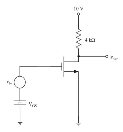
(a) Calculate  $V_{DSQ}$  when  $V_{GSQ} = 1.5$  V (15 pts).
