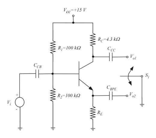
(a) Determine the proper value for  $R_E$
