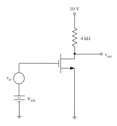
(a) Calculate  $V_{DSQ}$  when  $V_{GSQ} = 1.5 \text{ V}$  (15 pts).
