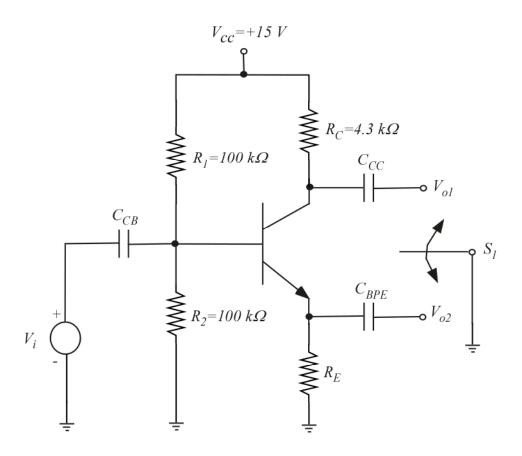
(a) Determine the proper value for  $R_E$
